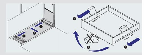
Using both hands, click on rail tabs (underneath drawer) and pull out and up simultaneously.
