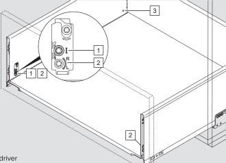
NOTE: Height, side and tilt adjustments must be achieved with a T20 Torx screwdriver
