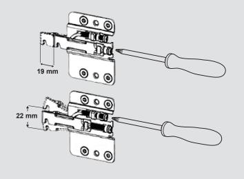
Hang cabinet and secure brackets into wall plates. Make sure to hear the brackets click into place.
