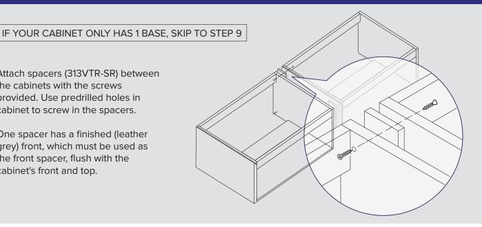
Copy steps 1-4 for each additional cabinet. Make sure to give the proper spacing between the spacer and the wall plate to consider the thickness of the cabinets frame.
